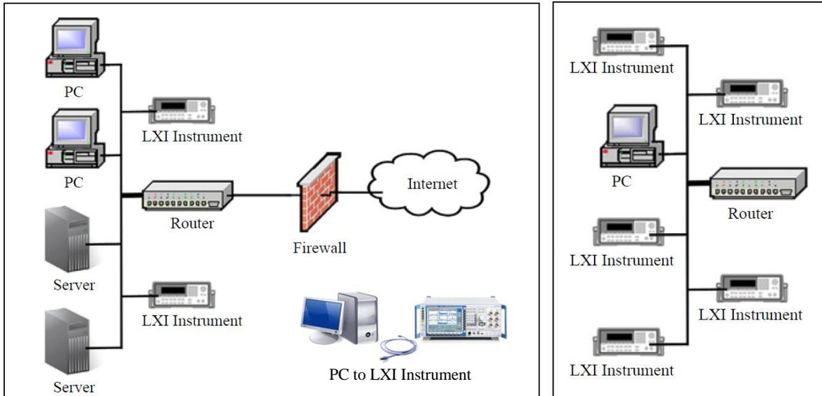
Sometimes it is preferred to create a private or isolated LAN, as in the upper right, where devices interconnect to each other but not to the Internet or any other networks by disconnecting the router from the Firewall and Internet. This keeps all outside traffic from interfering with the instrumentation and the test system computer. The test system computer, in this case, may be the only device connected to the company LAN, where developers can remotely login to develop tests.
