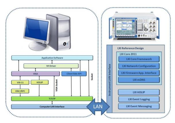
Modules in the shaded region encompass the base or Core set of features provided by the LXI Reference Design. These are required by every LXI Device to be LXI conformant.
