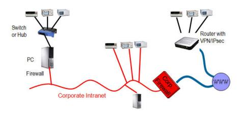
Even if your equipment is isolated from the wider LAN to a cell or lab, IP addresses are still required. Your IT department can advise on the correct range of IP addresses to use so that everything will work as expected.
