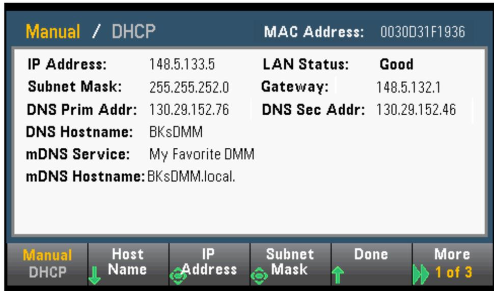
**Figure 7. Example Front Panel Configuration Page**
