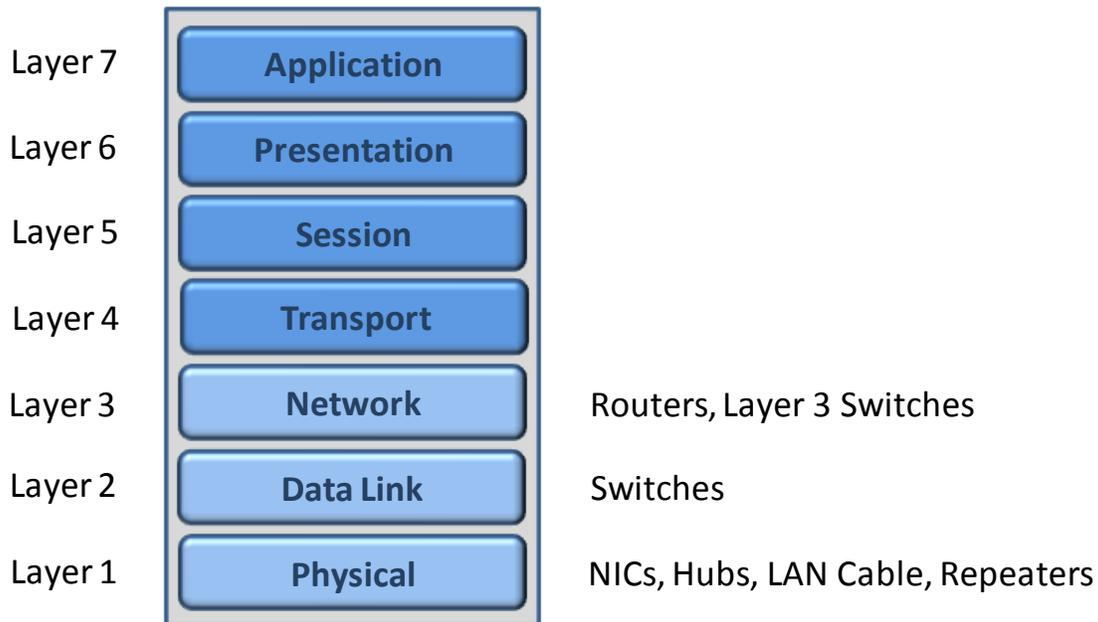
**Figure 2. OSI Model - Network Layers and Components**
