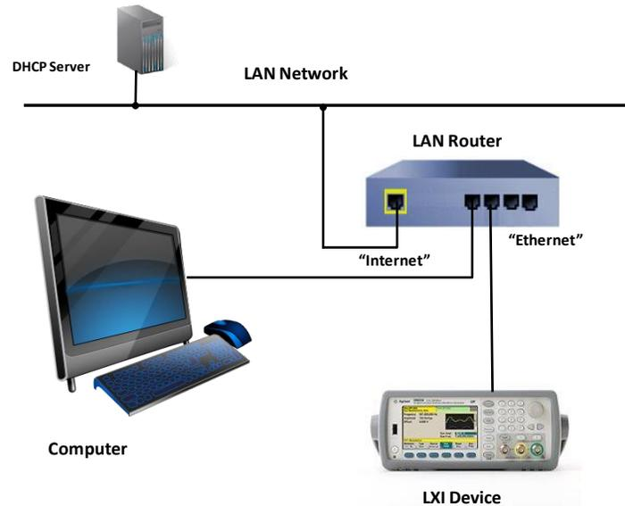
**Figure 6. Isolated System Configuration using a LAN Router**
